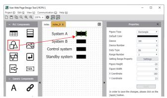
**1.** Drag the figure display of PLC Components to the design window.
