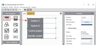
**1.** Drag the data block in PLC Components to the design window.
